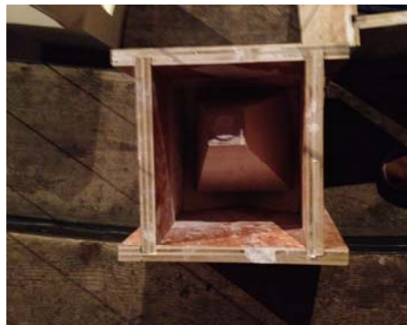
Mold with negative inset element
