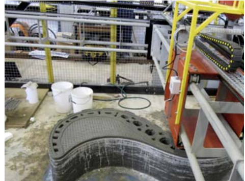
2. Wall element in production
