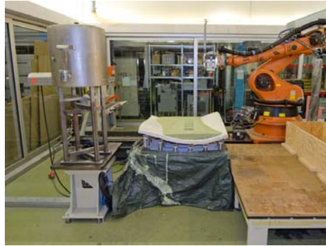
1. Production of wax molds with pin system
