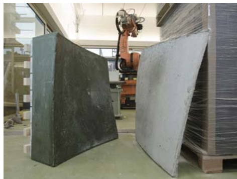
5. Thin concrete panel and wax mold
