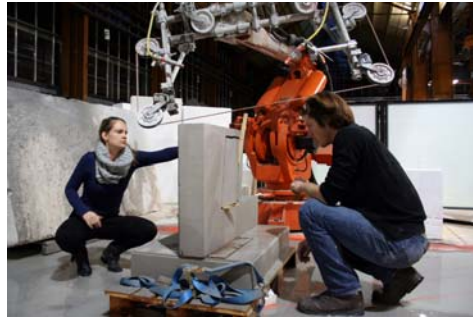
1. Robotic diamond wire cutting in process
