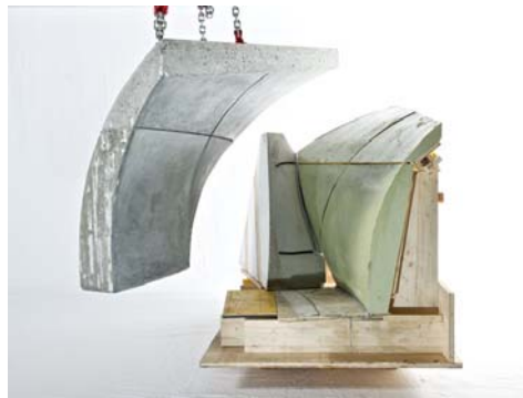
3. Concrete element and wax formwork
